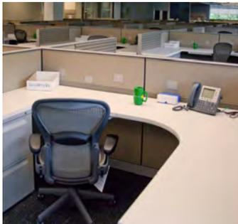
Keep office cubicle partitions no higher than 48 inches to allow for greater efficiency and more comfortable light levels.
