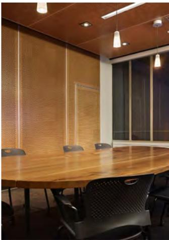
Meeting rooms have a target horizontal illuminance (average maintained fC) on the work surface of 45-55 fC for paper task performance. Vertical illuminance of 20-30 fC should be provided on selected display walls
